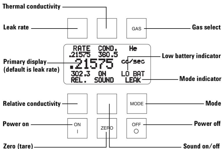
**Figure 4** Leak detector mode screen/buttons
