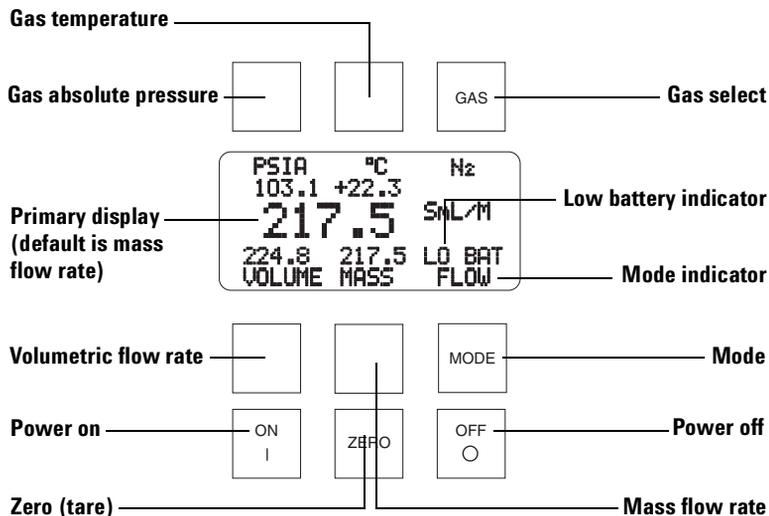
**Figure 2** Flow mode screen/buttons
